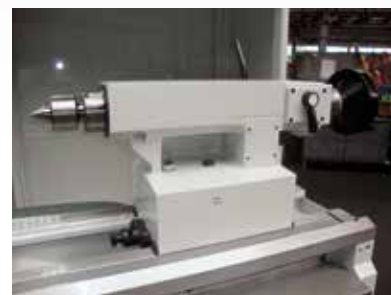
Tailstock with coupling to bed slide and 1:1 and 1:4 reductions for movement of quill
