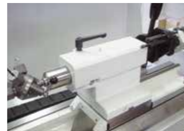
Boring quill with lever for tailstock
