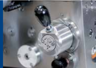
Single-lever control with safety locking
