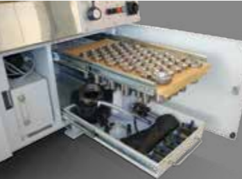
Machine base with detachable chip pan and lockable tool cabinet for accessories
