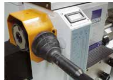
Lever-operated quick acting-collet attachment
