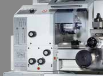
Headstock with back gear control for high torques
