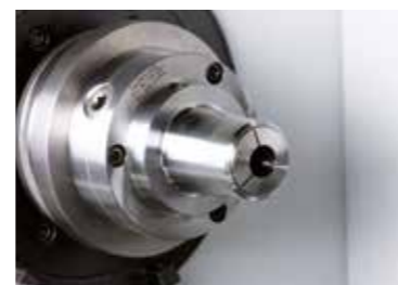
Hand-operated collet chuck
